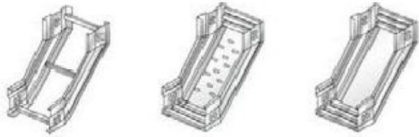
CN-QGQJ-DT1, -DPI, -DC1, -05型式大跨距垂直下弯通桥架 Large-span Vertical Down Curved way Bridge Frame
