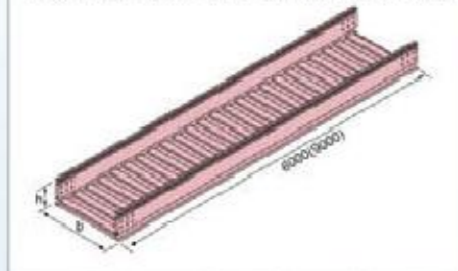
WQ/QGQJ-DC2-01型槽式大跨距汇线双边桥梁 Trough Large-span Cable Collection Bridge Frame
